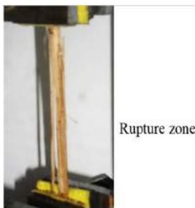
Figure 8: illustration of the rupture of a specimen
